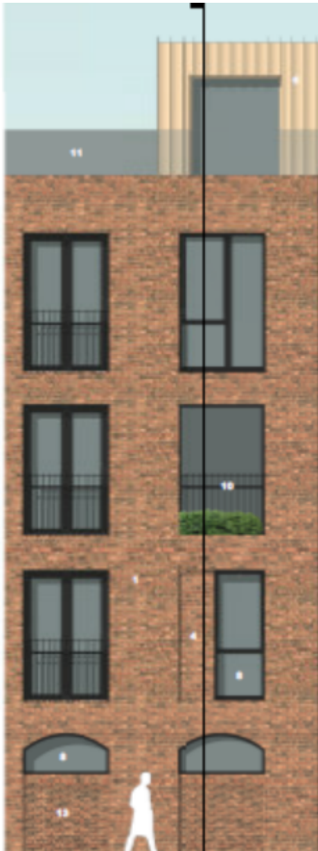
Bay study showing main façade to the towpath including brick work, recessed balcony and ceramic cladding together with brickwork detailing to the ground floor
